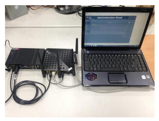
**Step1.** Connect the power, HDMI (recommended) or VGA and LAN cables of the signage box.
