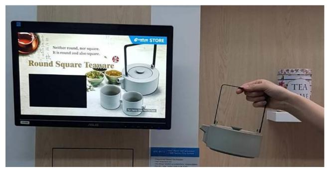
**Step16.** Fix the Sensor on the relevant advertising items and test the playback.
