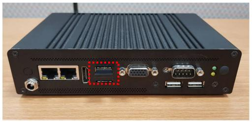
**Step2.** Plug Bluetooth dongle into USB port and turn on the signage box.
