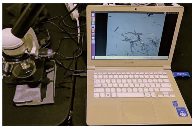
Image 2 and 3: WPIg enginner actual test by using Intel® NCS 2 for water quality detection
